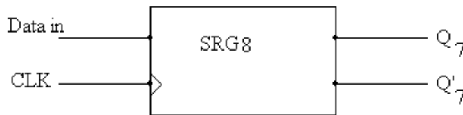
Fig(88): an 8-bit serial in/ serial out shift register.
